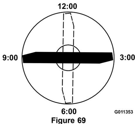
5. Rotate the marked end of the blade to the 3 and 9 o'clock positions (Figure 69) and measure the heights.
